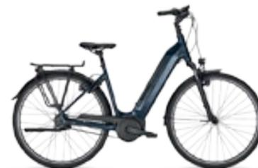
MOTOR: Bosch Active Line Plus, 36 V / 250 W / 50 Nm
